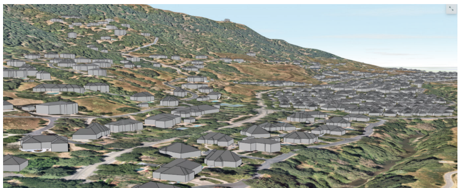
Example digital twin model from aerial imagery and AI-extracted buildings
