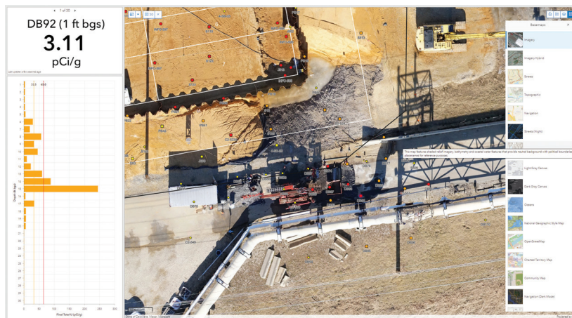
Drone images and data captured in biweekly flights were routinely imported into ArcGIS in a near-automatic process.
